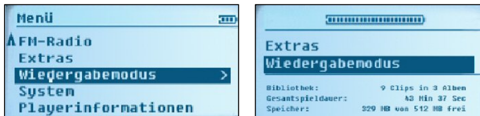
Figure 6.1: Variations of information presentation used in the study (high usability left, low usability right).
